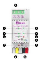
A. Supply voltage terminals B. Reset button C. Programming button D. Aux output connector E. KNX TP connector 1. LED input voltage  $V_{\text{N}}$  2. LED bus voltage  $V_{\text{BUS}}$  3. LED telegram traffic 4. LED output current  $I_{\text{OUT}}$  5. LED internal temperature 6. LED KNX reset 7. Programming LED
