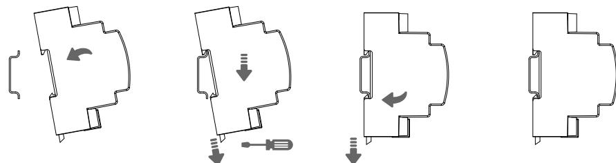
Removing from DIN rail
